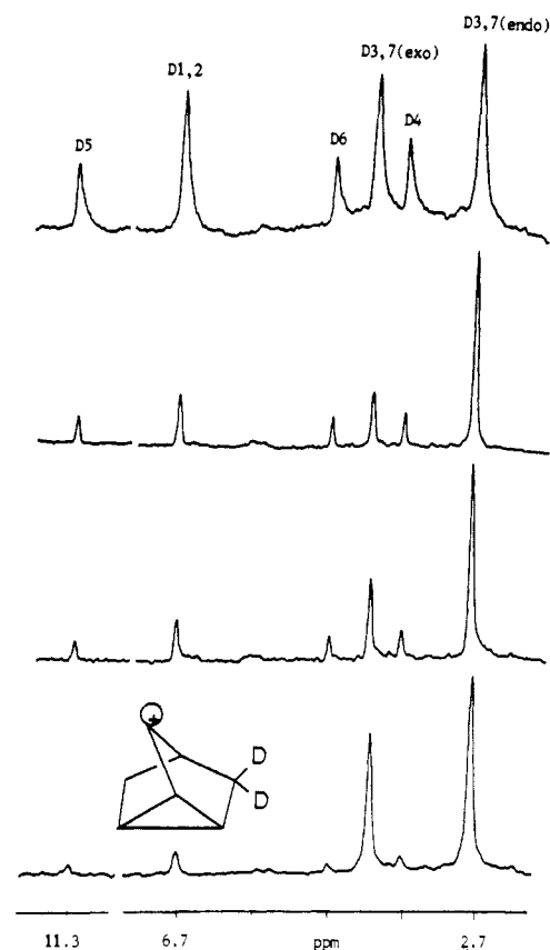
Figure 1. 2 H NMR of 3,3-dideuterionortricycyl-5-yl cation as a function of increasing sample temperature: bottom, –80 °C; middle, –45 °C over time (70 min); top, 0 °C.
